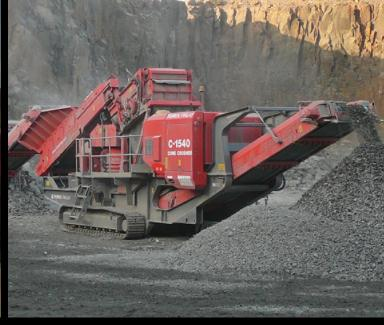
The Terex Finlay C-1540 tracked mobile cone crusher has a proven pedigree in aggregate and ore surface mining applications. This efficient and productive machine incorporates the proven Terex® 1000 cone crusher with direct variable hydrostatic drive, automatic tramp relief and hydraulic closed side setting (CSS) adjustment.
